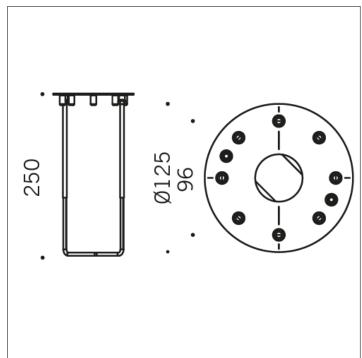
S.5680 ANCHOR FLANGE TO BE CEMENTED TO THE GROUND
