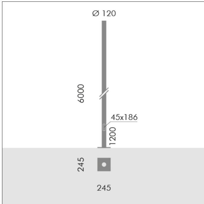
**S.2848****H 6,0m Ø120mm CYLINDRICAL POLE WITH BASE**
