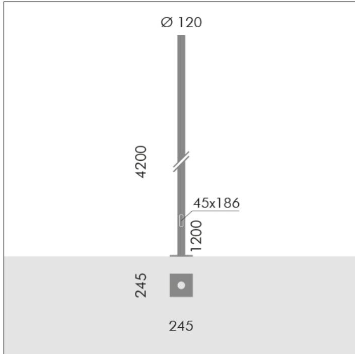
**S.2846****H 4,2m Ø120mm CYLINDRICAL POLE WITH BASE**
