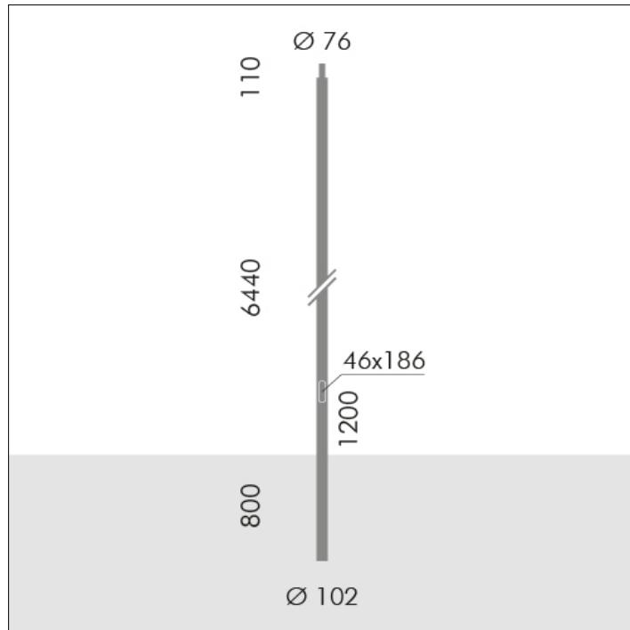
**S.2818****H 6,44m Ø102mm CYLINDRICAL POLE TO BE BURIED
